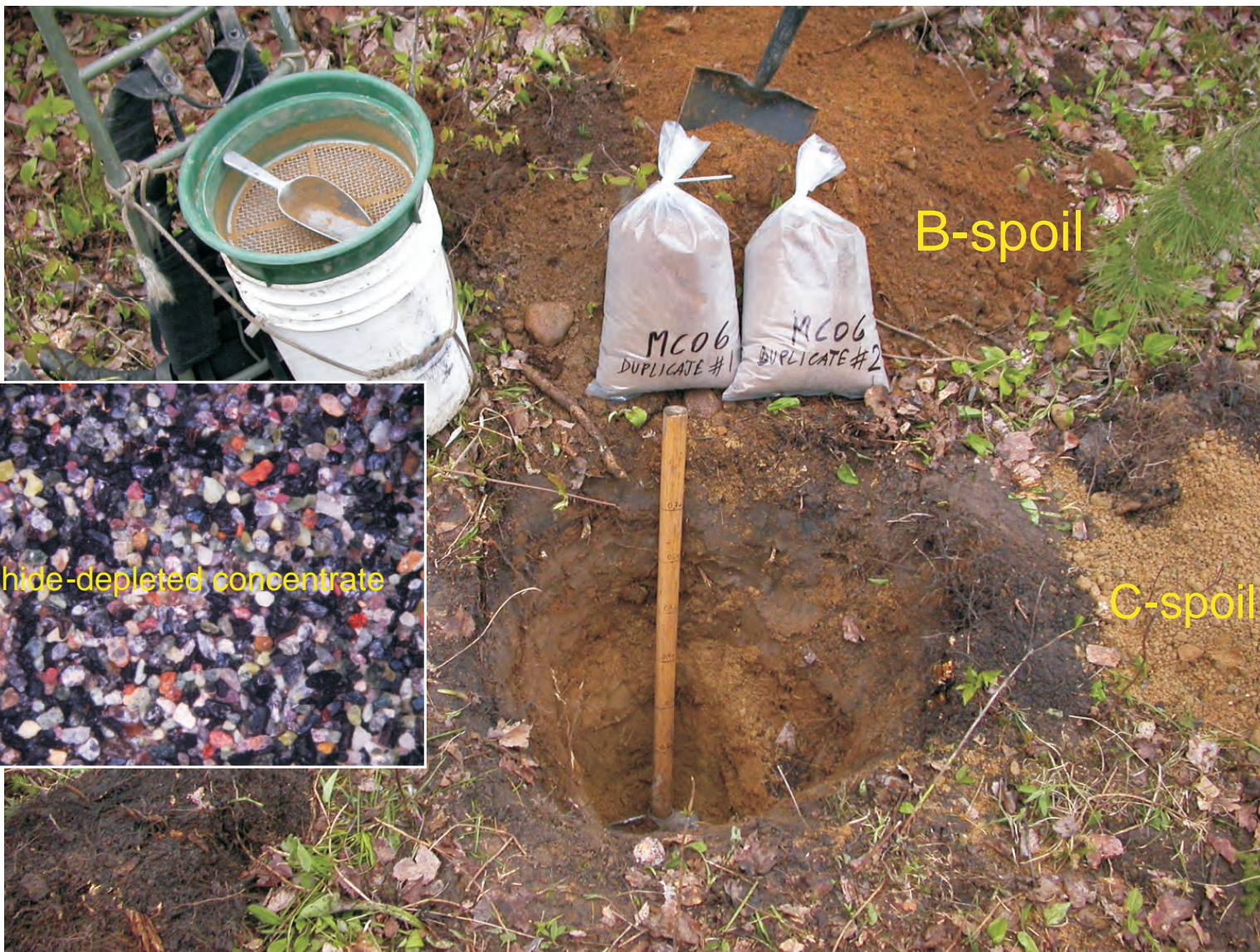
Figure 4 - (A) Typical till sample pit in non-permafrost terrain. The sample is normally collected at a depth of 0.5 to 1 m from the C-horizon of the soil profile which is less oxidized than the overlying B-horizon but still depleted of sulphide minerals as illustrated by the extracted heavy mineral concentrate (B). At this site, duplicate 10 kg samples of sieved till matrix were taken for quality control. Source: ODM archives.
